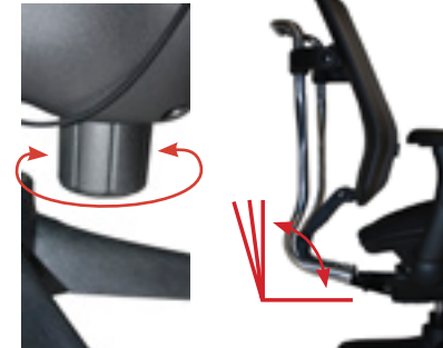
Backrest Tilt Tension Adjustment Twist knob under seat to adjust backrest tension. Twisting clockwise increases tension.
