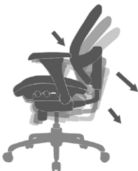
KNEE TILT Chair's pivot point is located closer to the front of the seat.
