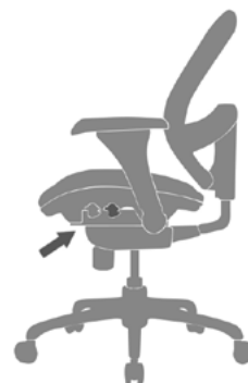
TILT LOCK Lock the chair's tilt mechanism to retain an upright position.
