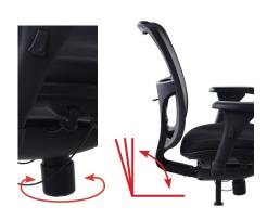
**BACKREST TILT TENSION ADJUSTMENT**Twist knob under seat to adjust backrest tension. Twisting clockwise increases tension.
