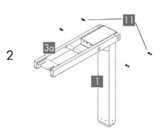
Place one of the Legs (part 1) into the Frame End-CB (part 3a) ensuring that the bar (arrow) is on "top" in relation to the Leg (part 1).
