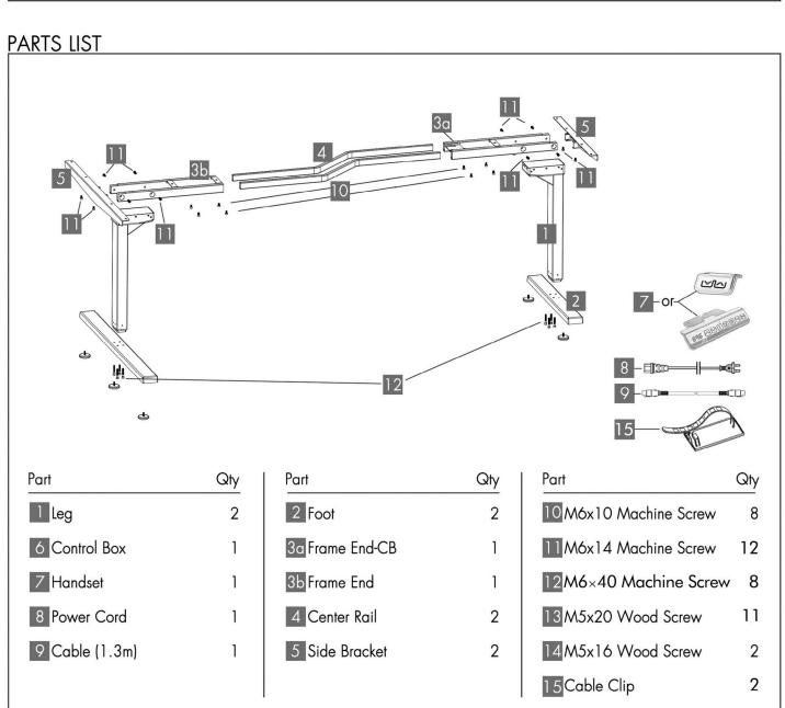
Lay out all components and hardware to ensure that you have all the components and hardware listed on the parts page. Slide the Control Box (part 6) off the Frame End-CB (part 3a) and set aside. Fully separate Frame End (part 3b) from Frame End-CB (part 3a). You will find the Center Rails (part 4) inside.
