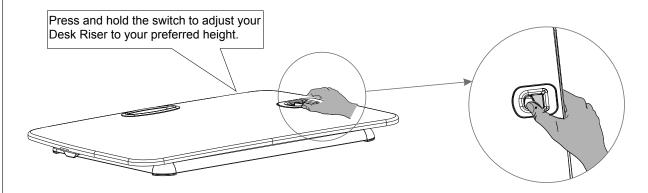
To raise your Desk Riser, press and hold the switch on the surface with your thumb, then lift the Desk Riser while holding both sides of the work surface. Let go of the switch and your Desk Riser will lock into place. To lower your Desk Riser, press and hold the switch on the surface with your thumb, then press down on the Desk Riser while holding both sides of the work surface. Let go of the switch and your Desk Riser will lock into place.
